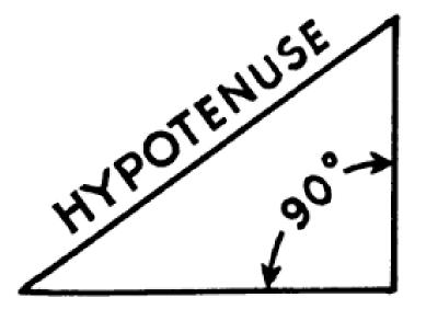
Pythagorean Theorem – in a right triangle, the sum of the squares of the lengths of the legs is equal to the square of the length of the hypotenuse; if <u>a and</u> <u>b are legs</u> and <u>c is the hypotenuse</u>.
